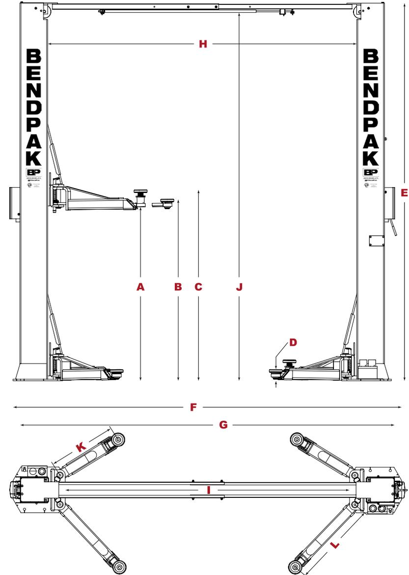
\*Optional bolt-on top extension for columns raises the overall height and overhead safety bar an additional 24". Must be ordered from BendPak at time of order.
